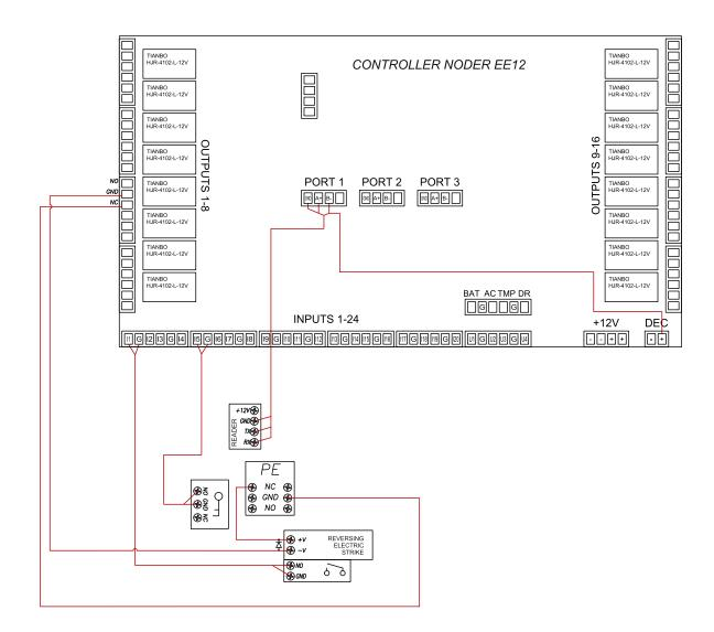
If it is necessary to use a collective button, connect the power supply of all reversing electric strikes to one module and, similarly to the above, break the power supply of the entire module with the collective buton.
