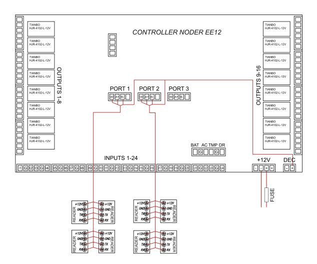
Value of protection should be adjusted to the number and power of connected readers. The protection used must not exceed 2A.
