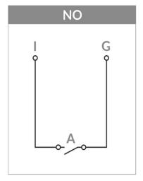
Input configured as NO is used for the exit button. After pressing it, the relay is activated and the event "Opening by exit button" is received.
