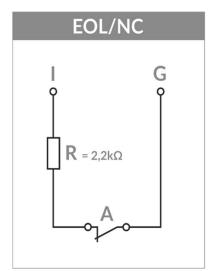
Detector in configuration with end of line resistor (2,2kOhm). Opening the circuit triggers an alarm. We do not receive information about sabotage ("Alarm" event is generated) and receive about fault ("Fault" event is generated).
