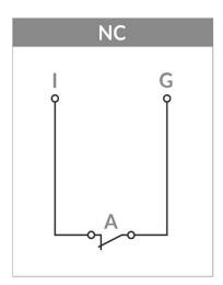
Detector with normally closed output. Opening the circuit triggers an alarm. We do not receive information about sabotage ("Alarm" event is generated) or fault ("Alarm" event is not generated).
