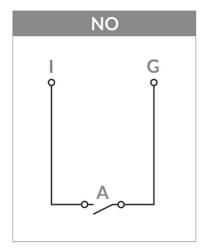
Detector with normally open output. Closing the circuit triggers an alarm. We do not receive information about sabotage ("Alarm" event is not generated) or fault ("Alarm" event is not generated).
