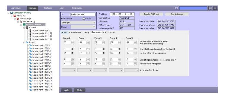
The controller can handle 5 card formats based on number of received bits. Intellect gives you the choice of predefined card formats or their manual configuration.
