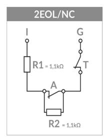
Detector in configuration with 2 end of line resistors (2x1,1kOhm). Opening the circuit triggers an alarm. We receive information about sabotage ("Tamper" event is generated) and ("Fault" event is generated).
