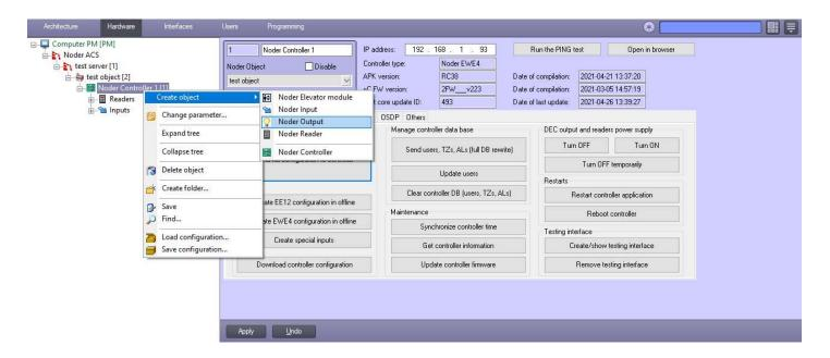
Object can be used in an Intruder Alarm System (after created, it will be visible in IAS Zone settings) to be activated on alarm or just to control relay from map, macro or script.
