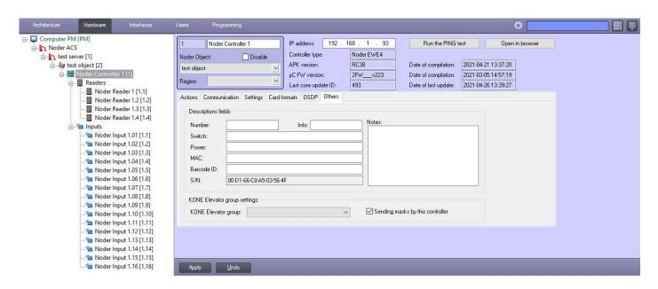
**Descriptions fields** – information about the network and electrical infrastructure can be stored. You can record the switch and socket number, electrical switchboard and fuse, MAC controller address, and more. The information stored **does not affect the logic of the controller**.
