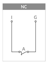
Input configured as NC is used for the door sensor or emergency exit button. Door sensor informs about the current status of the door. After pressing emergency exit button event "Emergency exit button pressed" is received
