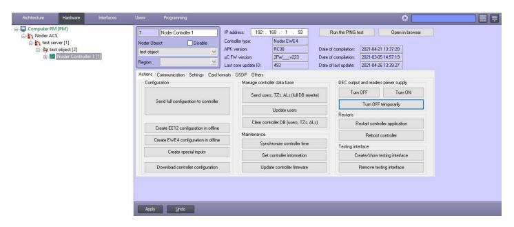
After adding the **Controller object**, configuration interface is displayed. In the **IP adress field** enter previously set controller IP address and click *Apply* to send changes. *Run the PING test* runs cmd.exe and monitors the device with the ICMP protocol. *Open in browser* will launch the default web browser in the system and automatically log on to the controller's website.
