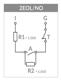
Detector in configuration with 2 end of line resistors (2x1,1kOhm). Closing the circuit triggers an alarm. We receive information about sabotage ("Tamper" event is generated) and ("Fault" event is generated).
