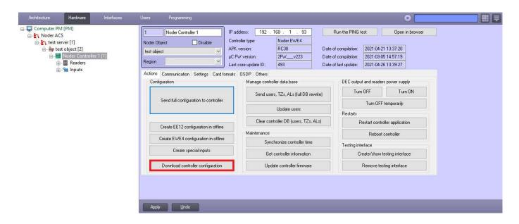
After downloading the configuration from controller will be created *Inputs* and *Readers*. 12 readers and 20 inputs will be crated for EE12 and 4 readers and 16 inputs will be crated for EWE4. It is necessary to configure readers and zones according to the needs of the system. **Unused ones to be removed and then send the configuration to controller** (button "Send full configuration to controller").
