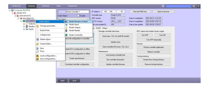
After choose the object, a window will open in which you should assign a number and name the device. Click Apply, a window of module options will appear.
