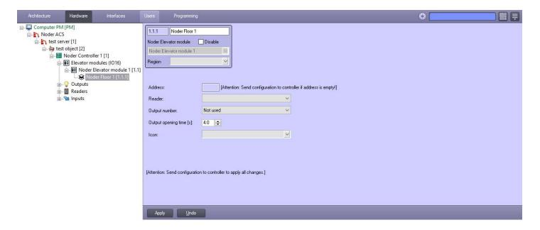
**Reader** – a physical reader in the elevator, to which the module relays are activated when an authorized card is put to device. The reader should be assigned to all floors it serves. After applying the authorized card, the relays are activated according to the access level assigned to the user.
