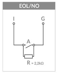
Detector in configuration with end of line resistor (2,2kOhm). Closing the circuit triggers an alarm. We receive information about sabotage ("Tamper" event is generated) and do not receive about fault ("Alarm" event is generated).
