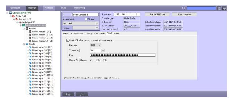
**Use OSDP v2 protocol to communication with readers** – selecting this function allows to use OSDPv2. Otherwise, communication with the factors will follow the **RS485** protocol. OSDP v2 options:
