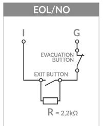
Input in configuration NO with end of line resistor (2,2kOhm). After pressing exit button, the relay is activated and the event "Opening by exit button" is received. After pressing evacuation button, the event "Emergency button is pressed" is received.
